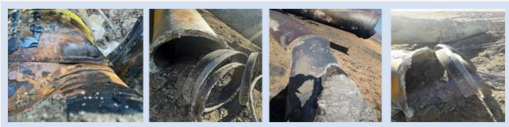
Figure 18: Post-earthquake pipe damages at RMS-A outlet
